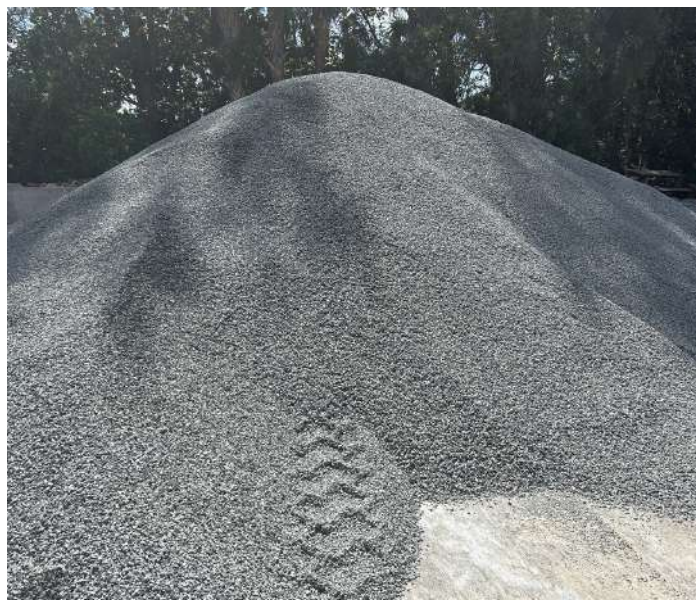
Quality control testing of gravel stockpiles onsite is important. Gravel should not be installed in a green cavity until it passes a QC test.
